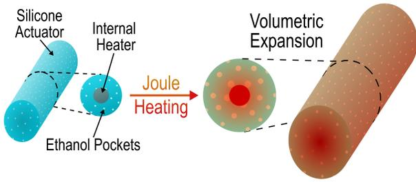
Fig. 2. All-soft actuator operation. Heating the core causes the external silicone to expand as the ethanol droplets trapped inside boil.
