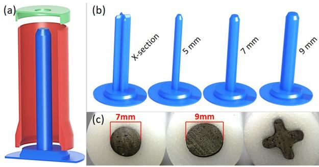
Fig. 5. CAD diagrams and photographs of the various heater core geometries. (a) A cut-away of the CAD rendering of the three-part mold. (b) Models of the four different cores used in the mold. (c) Cross-sectional photographs of three of the resultant heater core/actuator combinations.
