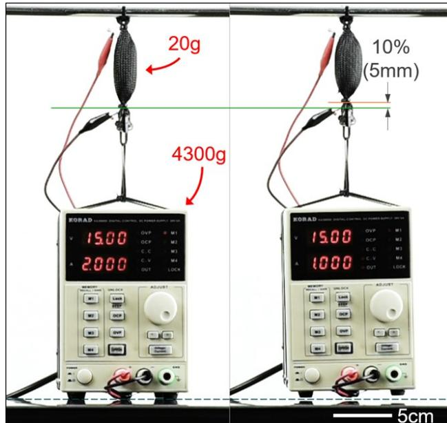
Fig. 1. All-soft heater/actuator being used as a McKibben-like muscle. The actuator is lifting its DC power supply, whose mass is greater than 200x that of the actuator.
