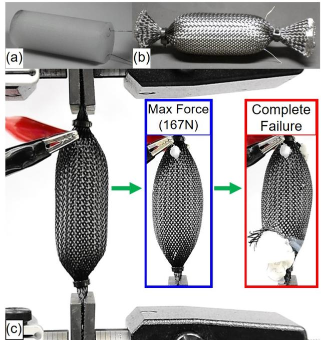
Fig. 7. Blocked force setup and test. (a) A Ni-Cr wire heated actuator. (b) The same actuator inside a mesh sleeve for use as a McKibben-like muscle. (c) The actuator installed in a blocked force test. Insets show the Joule heated actuator at its maximum force and then after complete failure (due to melting the external mesh).
